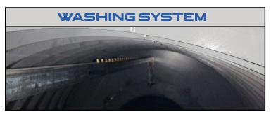
**Drum With Internal Screw** – Used where the drum angle is either level or a slight slope ie <5 deg. Level drums require an internal spiral to move the material through the drum. Sloped drums rely on the material moving through the drum by being rolled or lifted (by lifter bars) further down the drum each movement (or drop).
