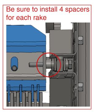
Once the brushes have been disassembled, mount thecombs, note the direction. Also don't forget to fit the 4 spacer bushings.
