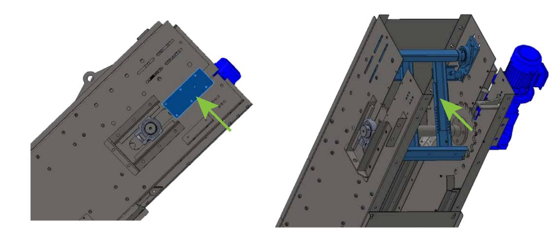
Connect the motor and rotate it to bring each brush to the height of the covers just removed (see 5)
