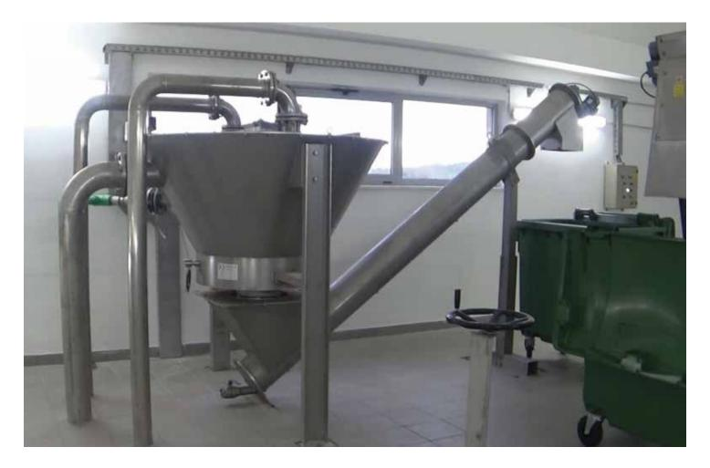
The CDL – GRIT WASHER is used for the separation of sandy materials contained in waste water, and for the simultaneous washing of the organic substances.
