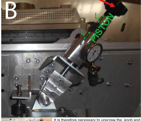
It is therefore necessary to unscrew the knob and reposition it as shown in photo B, then open the indicated cap / bolt, fill it with oil and then close it again.
